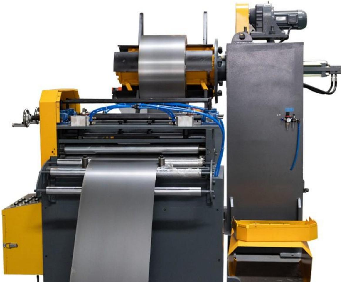
3. A folding device is installed at the front end of the leveling feed roller, and the movable roller is pulled by the air cylinder. When the material is fed for the first time, the material head is bent and flattened before being sent to the straightening machine.
